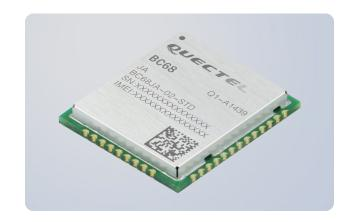
BC68 is a high-performance NB-IoT module which supports multiple frequency bands of B1/B3/B5/B8/B20/B28 with extremely low power consumption. The ultra-compact  $17.7 \, \text{mm} \times 15.8 \, \text{mm} \times 2.3 \, \text{mm}$  form factor makes it a perfect choice for size sensitive applications. Designed to be compatible with Quectel GSM/GPRS M66 module in the compact and unified form factor, it provides a flexible and scalable platform for migrating from GSM/GPRS to NB-IoT networks.
